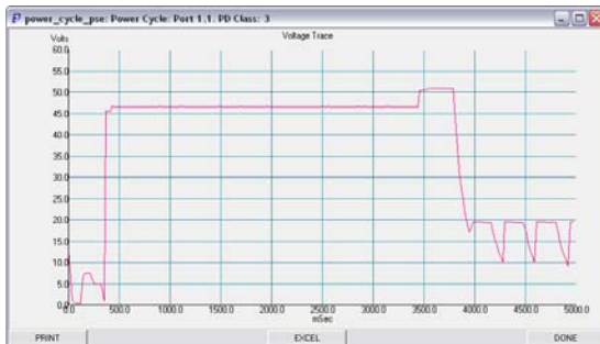
Figure 3.9: Power Up/Down Voltage Cycle
