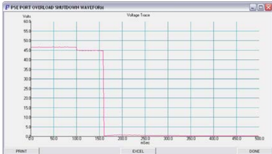
Figure 3.12: Disconnect Shutdown Voltage
