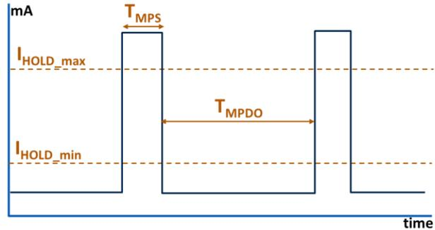
Figure 2.13 DC MPS Minimum Power State
