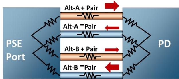
Figure 2.11 Pair-to-Pair Current Unbalance
