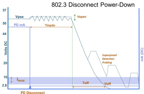
Figure 2.12 802.3 PoE Disconnect Power-Down
