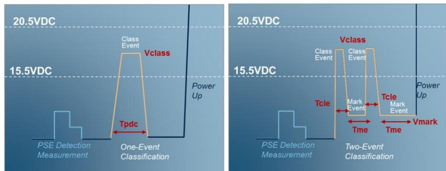
Figure 2.6 PD Classification under the 802.3at Specification
