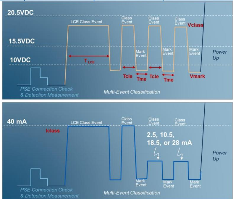
Figure 2.7 PD Classification under the 802.3bt Specification
