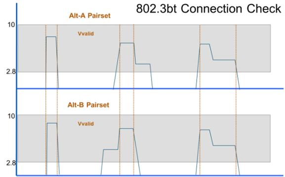
**Figure 2.5** 802.3bt Connection Check
