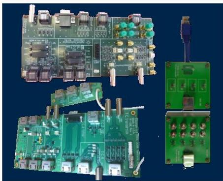
Figure 1.2 Ethernet PHY Test Fixtures
