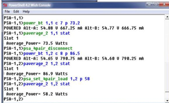
Class 7 4-Pair Power-Up and Shutdown on Port 1 followed by Class 8 Power-Up on Port 2
