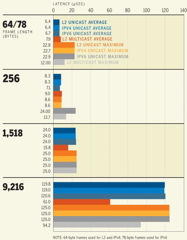
There was little variation in delay across different unicast test cases, indicating that the switch processes all flows the same way in hardware. Perhaps more significantly, latency is relatively low for a large Gigabit Ethernet modular switch.
