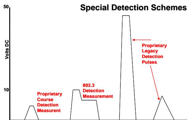
Figure 2.5 Hybrid Proprietary Detection Methods
