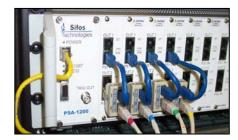
Sifos offers PSA RJ-45 Port Combiners and short Ethernet cables at no charge for those who wish to take advantage 802.3at pre-standard high power PoE testing and are using Conformance Test Suite.
