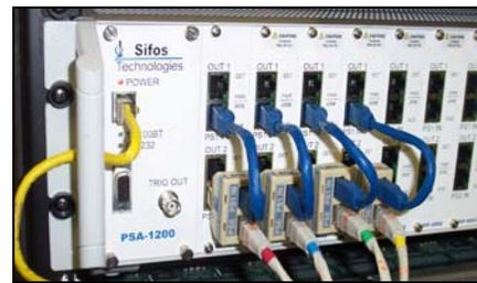
With the anticipated release of IEEE 802.3at expected in 2008, first generation high power devices and Power Sourcing Equipment (PSE) are currently in active development throughout the networking industry. High power PSE's with capability to deliver well in excess of the 15.4 watt requirement of IEEE 802.3af PSE's are becoming available ahead of IEEE standard.
