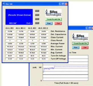
PDA Interactive allows instrument interactive control and report generation from a host PC connected via a serial interface port.
