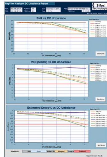
DC Unbalance tolerance is an extremely difficult assessment to perform. Sifos offers a unique solution that combines PowerSync Analyzer (or Programmable Load) ports with PhyView Analyzer test ports to produce fully automated analyses of the impact in varying levels of DC Unbalance to 100Base-Tx and 1000Base-T signal quality. Measurements include SNR (distortion), Low Frequency Response (attenuation) and Estimated Pulse Droop resulting from compromised magnetics.
