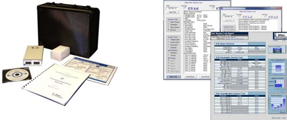
Sifos Technologies, Inc. ([www.sifos.com](http://www.sifos.com)) introduces the new PoE Service Analyzer that supports highly robust testing of both Type-1 (13W) and Type-2 (25W), including LLDP, PoE service at any PD connection point. The PoE Service Analyzer far surpasses PoE testing and interoperability analysis available in more common service testing devices.
